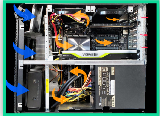
Example of airflow in BIMBOX versus a typical computer in an AEC firm
