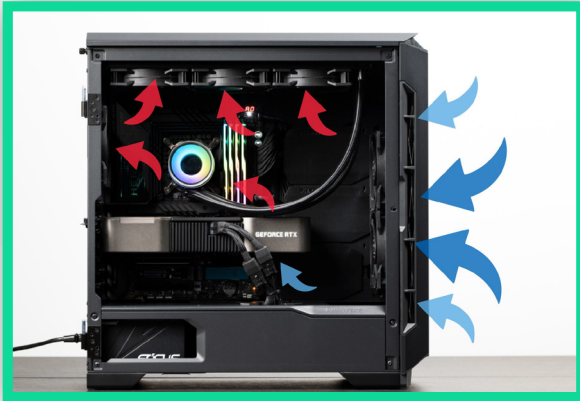
Example of airflow in BIMBOX versus a typical computer in an AEC firm
